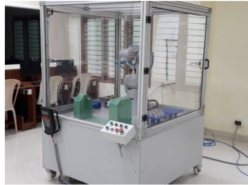
Industrial Robot Cell (Mitsubishi 6-axis Articulated Arm)
